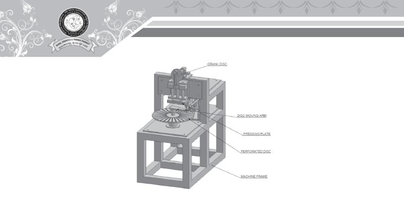
Design of Piston type Fish meat picking machine
